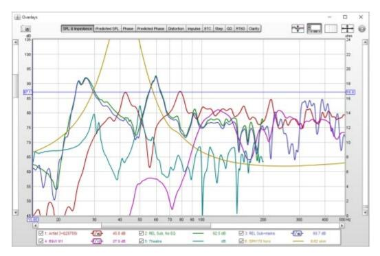
The overlays window shows plots for all the currently loaded measurements. It is shown by pressing the Overlays button in the toolbar of the main REW window.
