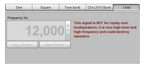
The jitter test signal consists of a square wave at one quarter of the sample rate at half full scale amplitude modulated by a square wave at 1/192 of the sample rate that alternates between 0 and -1 lsb at the 24-bit level. **This signal is NOT for replay over loudspeakers, it is very high level and high frequency and could destroy tweeters**. Note that Java drivers on windows only support 16-bit data and the OS adds dither on the input, so analysing the signal on Windows requires ASIO drivers.
