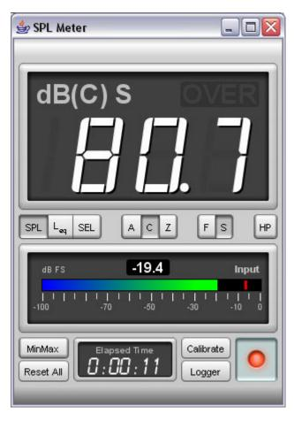
The meter displays either sound pressure level (SPL), time-average equivalent sound level ( $L_{eq}$ ) or sound exposure level ( $L_{E}$ ) according to the selection made on the buttons below the display. The SPL reading is filtered with either a "Fast" (125ms) or "Slow" (1s) time constant, selected via the F/S buttons. For general use the "Slow" setting is best. When the **HP** button is pressed a high pass filter is applied that eliminates content below approximately 8Hz.
