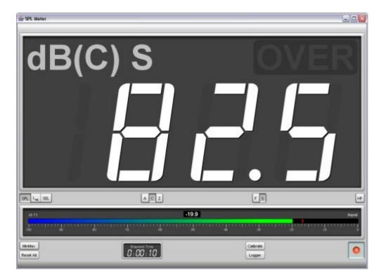
Below the main row of controls a level meter shows the current soundcard input level in dBFS, the peak is shown by the red bar while the numeric indicator and the coloured bar show the rms level.
