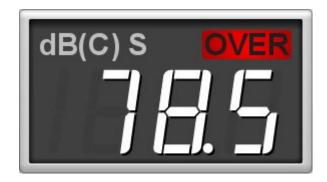
The SPL meter window can be resized as required, the main SPL display digits automatically scale to suit the available space. The meter can also be set to full screen.
