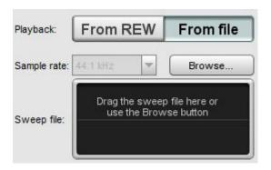
A <u>Measurement Sweep</u> file must be generated and <u>saved</u> from the REW signal generator. The sweep file must include the acoustic timing reference signal, REW uses that to synchronise input capture to playback
